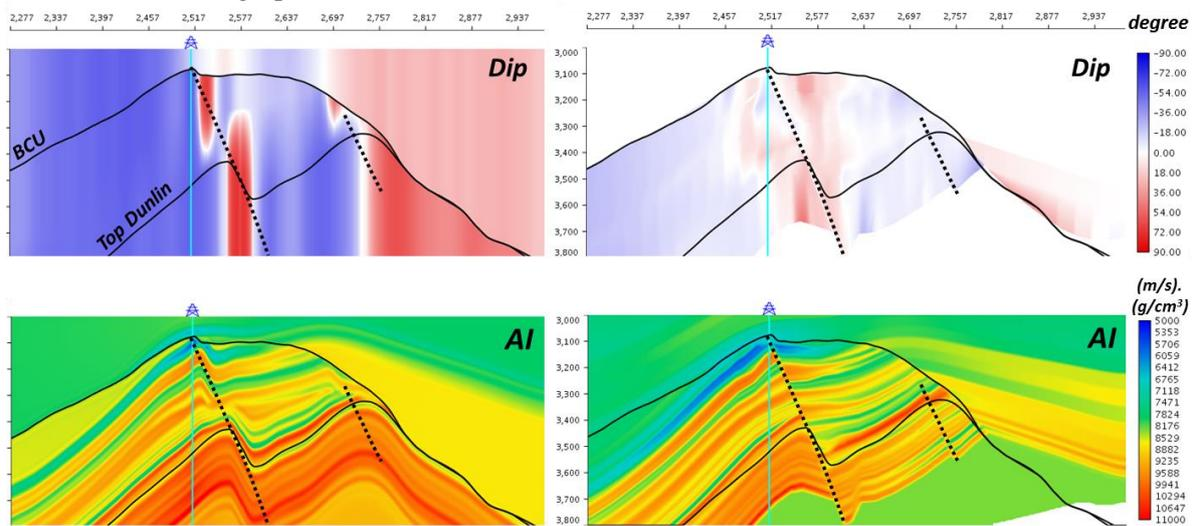
**Figure 1** InLine 2322 Dip associated to no-faulted *a priori* model (top left) and the faulted one (top right). Dip of stratification is respected between both sides of the faults (black dashed lines). Impedance from no-faulted *a priori* model (bottom left) and from the faulted one (bottom right.)
