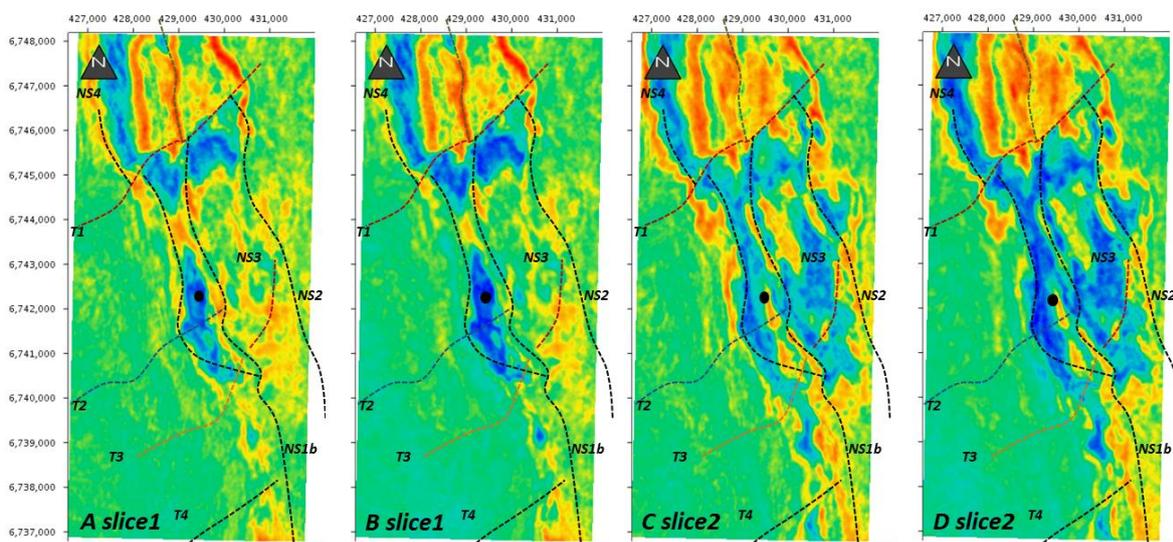
**Figure 4** Inverted impedance using no-faulted *a priori* model (A, C) and using a faulted one (B, D). One can note the better delineation of the TopBrent (blue colors) with inversion using the faulted *a priori* model (B, D). Slices A, B are at 3100 and slices C, D are at 3130.
