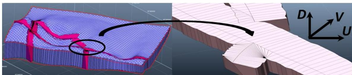
**Figure 2** The thick Cartesian grid (left) containing a geological unit in the depositional  $(U,V,D)$  domain. A zoomed area of the hexahedron mesh along part of the fault network (right).  $U$  and  $V$  are horizontal parametric coordinates and  $D$  is the geological age.
