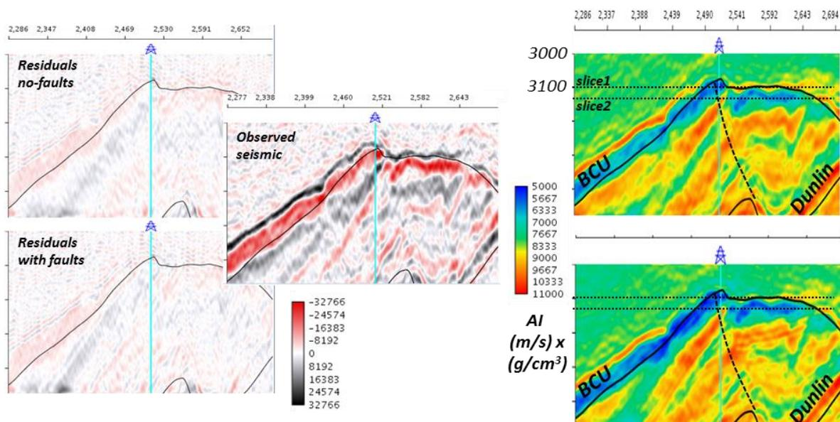
**Figure 3** Comparison of residuals (left) compared with the observed seismic (middle). Comparison of inverted Acoustic Impedance using a no-faulted *a priori* model (top right) and a faulted one (bottom right).
